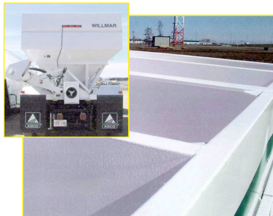
Right: Entire exterior box of sander (yellow & grey) is sprayed with LINE-X XS-100 .
