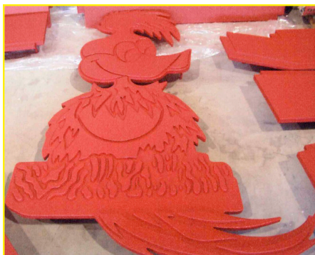
Above: MDF lettering and routed logo design coated with LINE-X.
